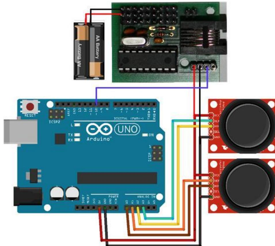
The Arduino Sketch is straight forward. The program would be reading each analogue input and compare the value acquired with the previous position. Would the values deviate from the previous reading then the Arduino would send the new position to the PiKoder/SSC. The Sketch [Four Channel Encoder for SSC \(.ino-Datei\)](#) can be downloaded here. This sketch is Open Source and is released under a [GNU General Public License Version 3](#).
