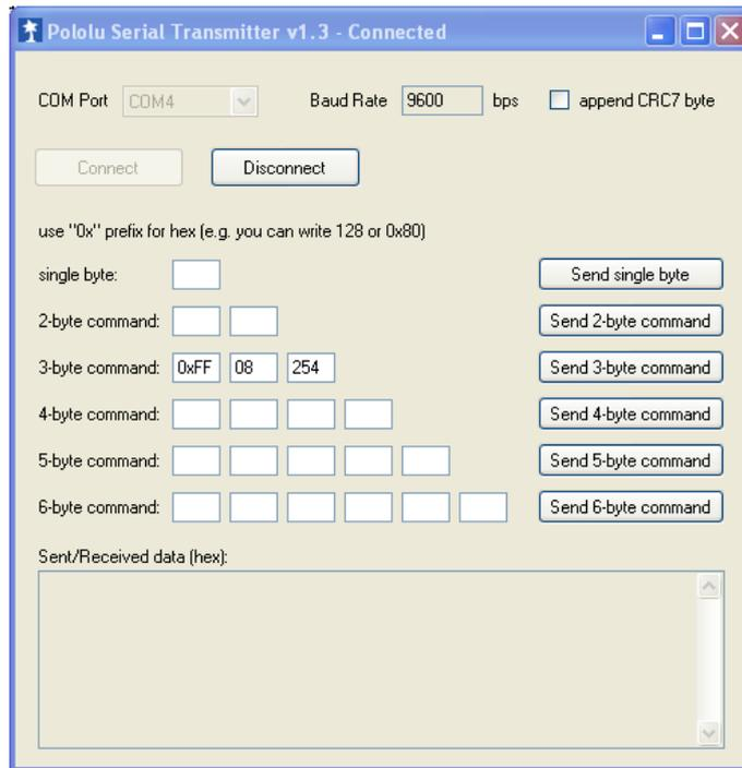
Once you hit the “Send 3-byte command”-button the bytes are sent to the PiKoder (see below); as per protocol definition there is no response by the SSC.
