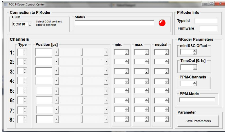
The PiKoder Control Center application would show COM10 to be the first available port in your computer. Select the COM port your PiKoder/SSC is connected to (in this example COM36, see below) and then click on the box to indicate your selection and communication to the controller will be established.
