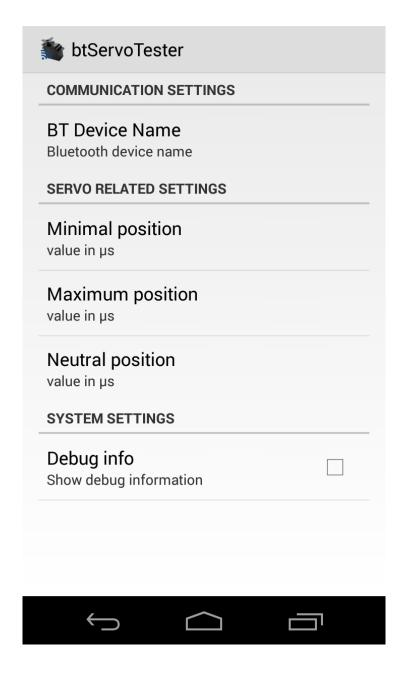
The default device name would be "HC-06" reflecting the PiKoder/SSC RX standard configuration. If you are employing another device then you can adapt the device name by tapping the field. Please note that the device which you are using has to be paired with your Android device.
